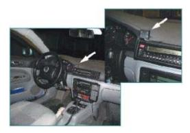
The camera can be installed near the rear view mirror, dashboard, etc. and a covert place like beneath seat for main unit, wireless siren (option) and wireless emergency switch (option).
