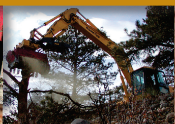
Double carbide cutting tips shred trees, stumps and shrubs to mulch
