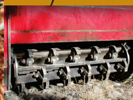
Double carbide cutting tips shred trees, stumps and shrubs to mulch
