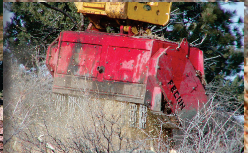
Double carbide cutting tips shred trees, stumps and shrubs to mulch
