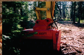
Double carbide cutting tips shred trees, stumps and shrubs to mulch
