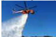
Helicopter "Water Drop" (250-2,500 gallons)
